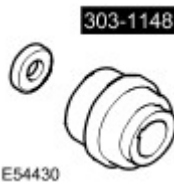
Installer oil seal front cover 303-1148
